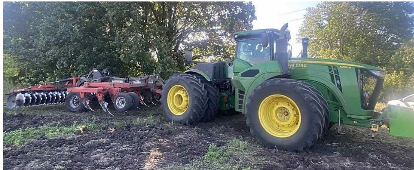
Fig. 2. John Deere 9470R + Gaspardo DIABLO-700 tillage machine
