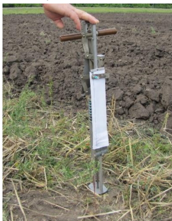
Fig. 1. Revyakin hardness tester for determining soil hardness
